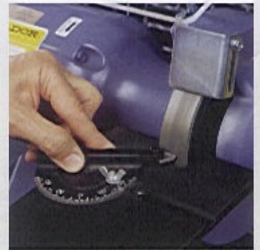
Compound angles are easy to set with the tilt table top and the sliding "T" protractor.
