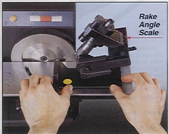
Serdi valve seat cutter with Accu-Finish in-the-cutter-body sharpening and adjustable rake angle. Other fixtures are available for Sunnen VSC/SGM and most popular ball driver seat cutters.
