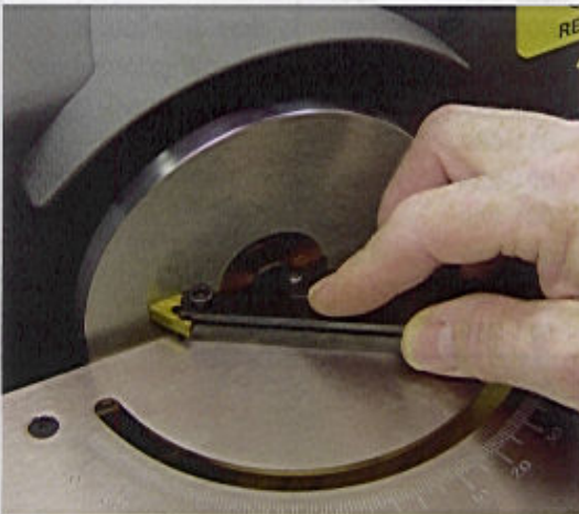
Built-in protractor and table angle insures accurate tool angles.
