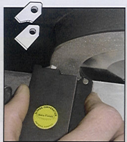
Sharpen Serdi-style bits on any Accu-Finish with this bit holder.
